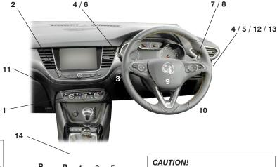
When parked, the electronic parking brake or handbrake should be fully applied with the vehicle left in first or reverse gear (manual transmission) or P (Park) for vehicles with automatic transmission
