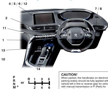
When parked, the handbrake (or electronic parking brake) should be fully applied with the vehicle left in first or reverse gear for vehicles with manual transmission or P (Park) for vehicles with automatic transmission.
