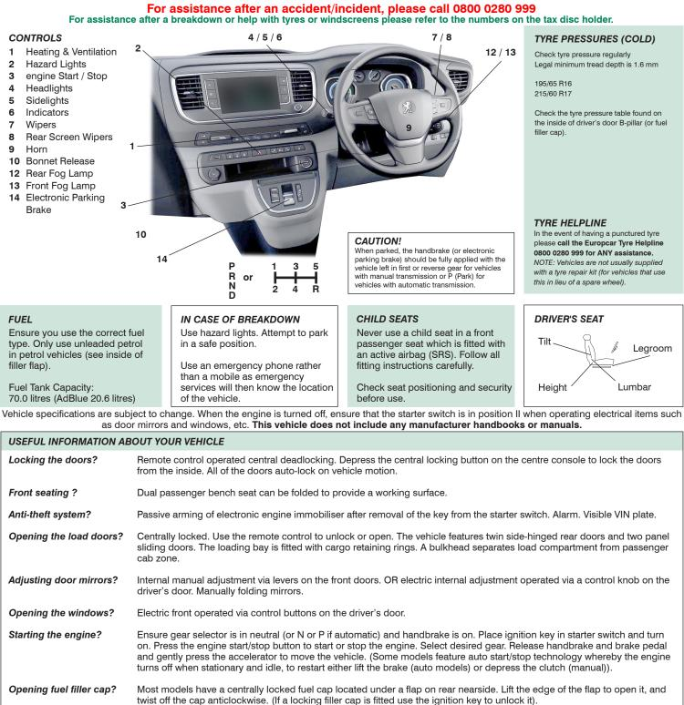
Releasing the bonnet? Pull bonnet release lever located on left hand side of front passenger footwell. Unhook catch under bonnet.
