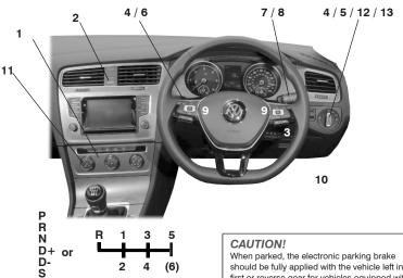
When parked, the electronic parking brake should be fully applied with the vehicle left in first or reverse gear for vehicles equipped with manual transmission or P (Park) for vehicles with automatic transmission
