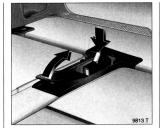
Push belt buckles into recess in floor and
