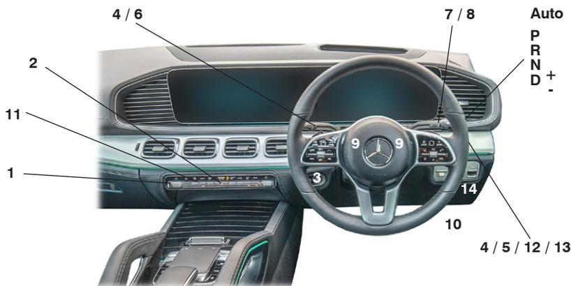
vehicle is fitted with a gear shift lever mounted on the steering column
