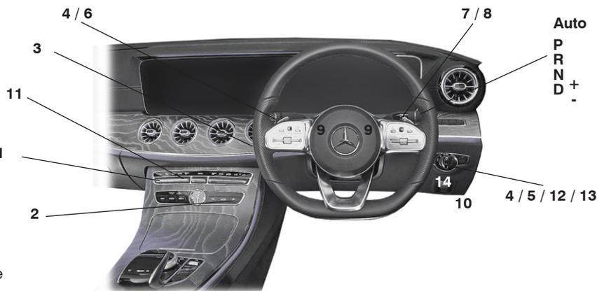
Vehicle is fitted with a dash mounted parking / hand brake, located on lower right of dashboard.
