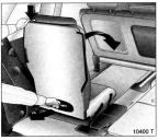
From luggage compartment, press button at top of seat backrest and push backrest forward. Raise seat by strap at rear and push backrest further forward until seat is lowered into vehicle floor.
