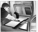
From luggage compartment, raise seat by strap and move it back until it locks audibly back into the upright position, supporting the backrest at the top with the other hand – see Fig. 9815 T.
