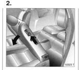
Folding down the seat backrest To facilitate entering and leaving the rear of the vehicle, the split rear seat backrest can be pushed forward. Pull up release lever and tilt seat backrest forward into second locking position.
