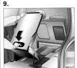
Open the cover in the floor between the seats and draw out the belt buckles Fig. 9813 T.
