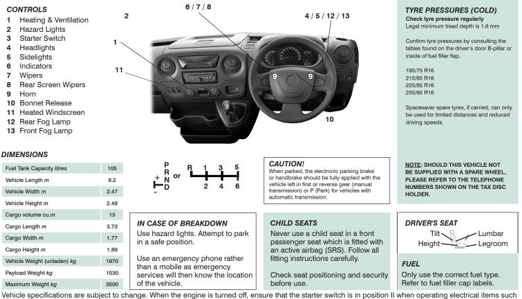
Vehicle specifications are subject to change. When the engine is turned off, ensure that the starter switch is in position II when operating electrical items such as door mirrors and windows, etc. This vehicle does not include any manufacturer handbooks or manuals.
