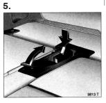
Push belt buckles into recess in floor and Installing luggage compartment cover \*
